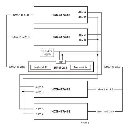
Figure 2. Recommended Network Setup for 220 Type Shelves
